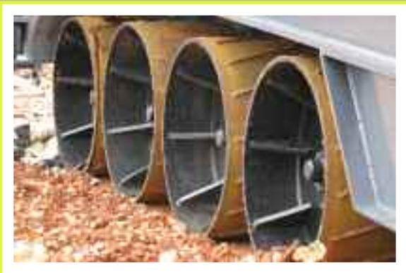
**Steel Wheels** in lieu of the standard rubber tires protect the tipper from fire and flats.
