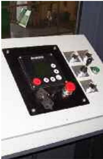
**Control Panel** that is simple to use and easy to maintain. Includes features such as engine auto-throttle and deck anti-jog. Operator's cab mounts to driver side of tipper frame.
